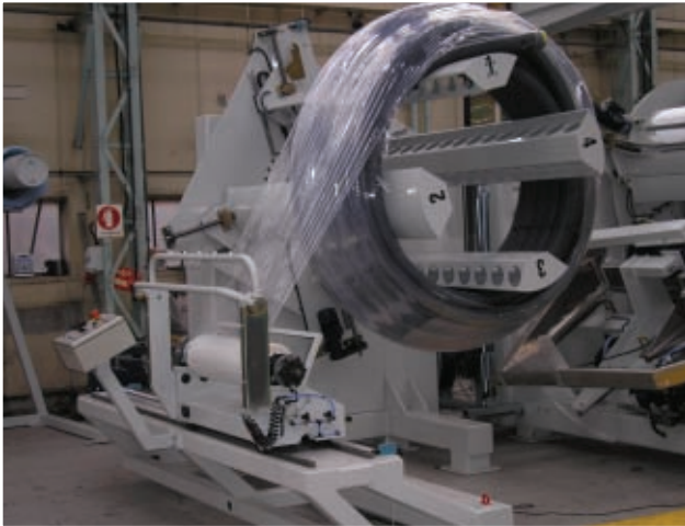
Secondary coiling stations for application of film or protective coatings
